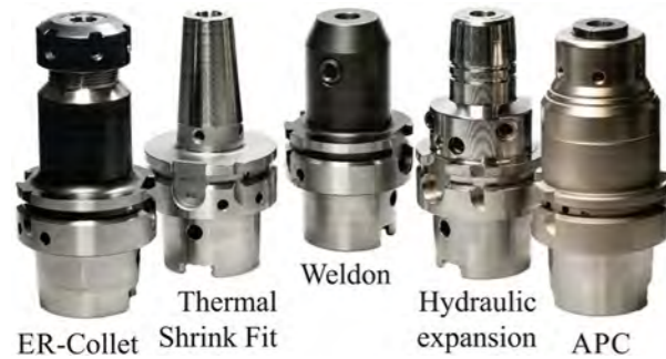
Fig. 1 Examples of the investigated tool holder systems
